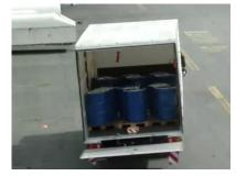
Static inclination test DIN EN 12195-1 Inclination angle: 45 degrees Inclination duration: 10 minutes Result: no displacement > 2 cm
